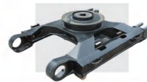
lower frame of excavator
